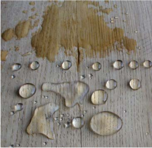
Figure 2: Wooden board test – upper half of the surface was left untreated while the bottom part was protected with the nanostructured coating.
