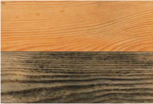
Figure 4: The durability test of pine board impregnation after 2 years: board protected with nanostructured coating (Top) and unprotected board (Bottom).
